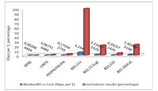
Figure 4: Bandwidth cost per technology
