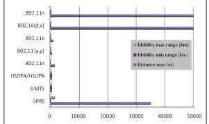
Figure 2: The protocol's range capabilities at a glance
